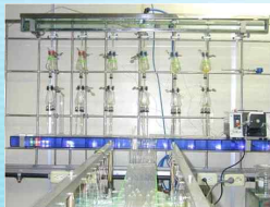
Continuous flow-through system supplying test solution
